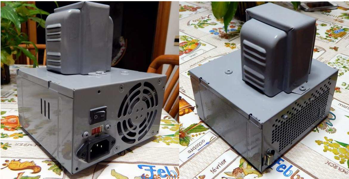
The anode voltage output can be adjusted with a trimmer between 200 and 280 Volts. I measured when loaded and it is well regulated at 280V up to 110 mA. Besides the voltage drops across the transformer and the change is reflected on the output.
